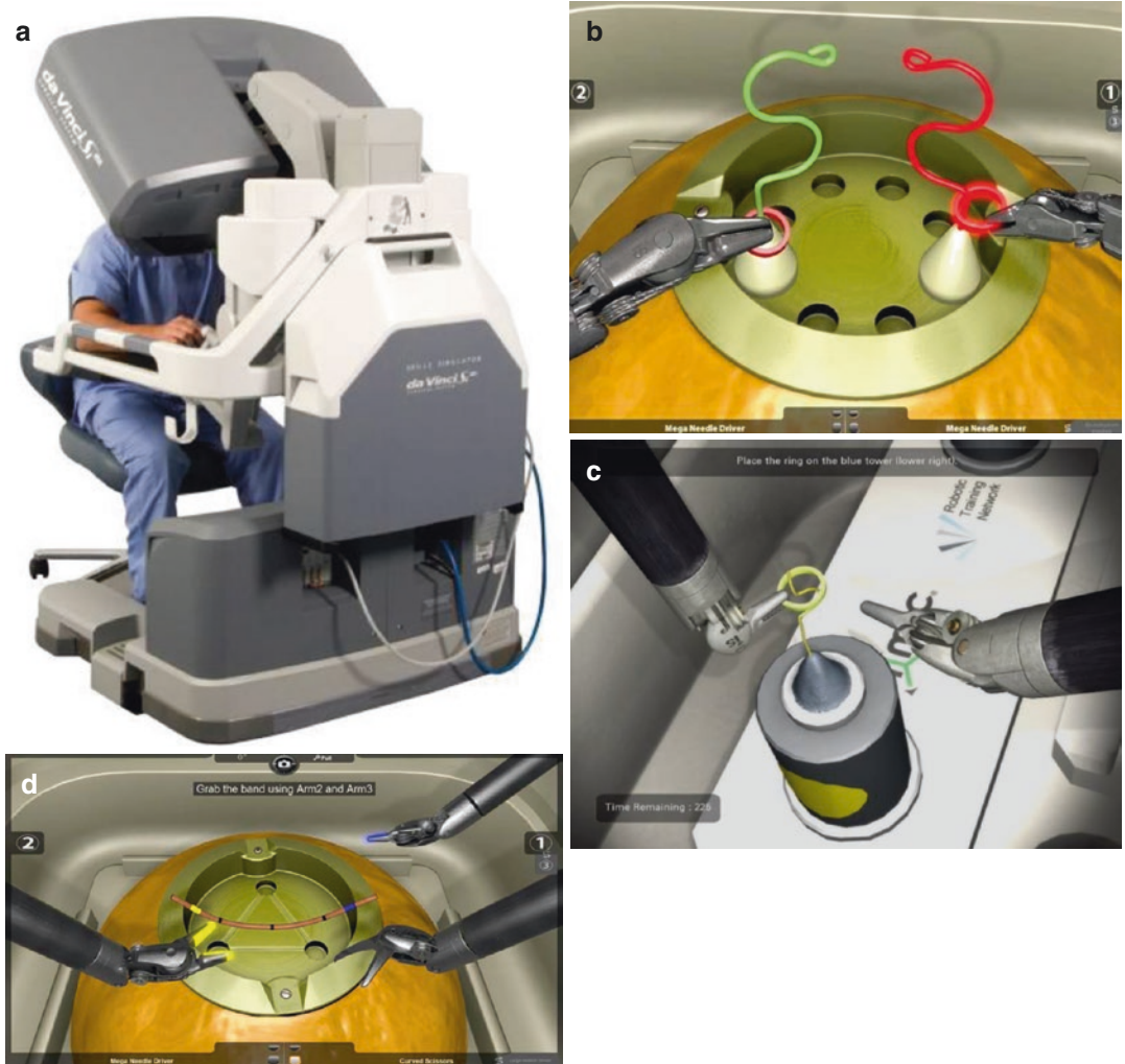
Fig. 16.6 da Vinci Skills Simulator® (dVSS) (a) and virtual reality simulation of the FRS dome: dVSS dome (b+c) with different skill testing units and RobotiX Mentor virtual reality simulation (d)
