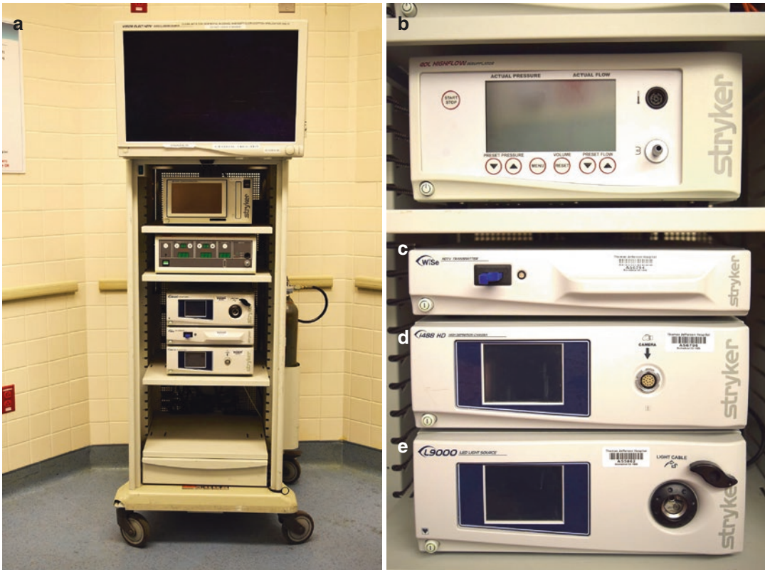
Fig. 2.18 Laparoscopic tower that includes the necessary hardware during a laparoscopic case. (a) Broad overview of components located on the tower. (b) Insufflator measures the pressure and the flow of gas that is provided dur-
